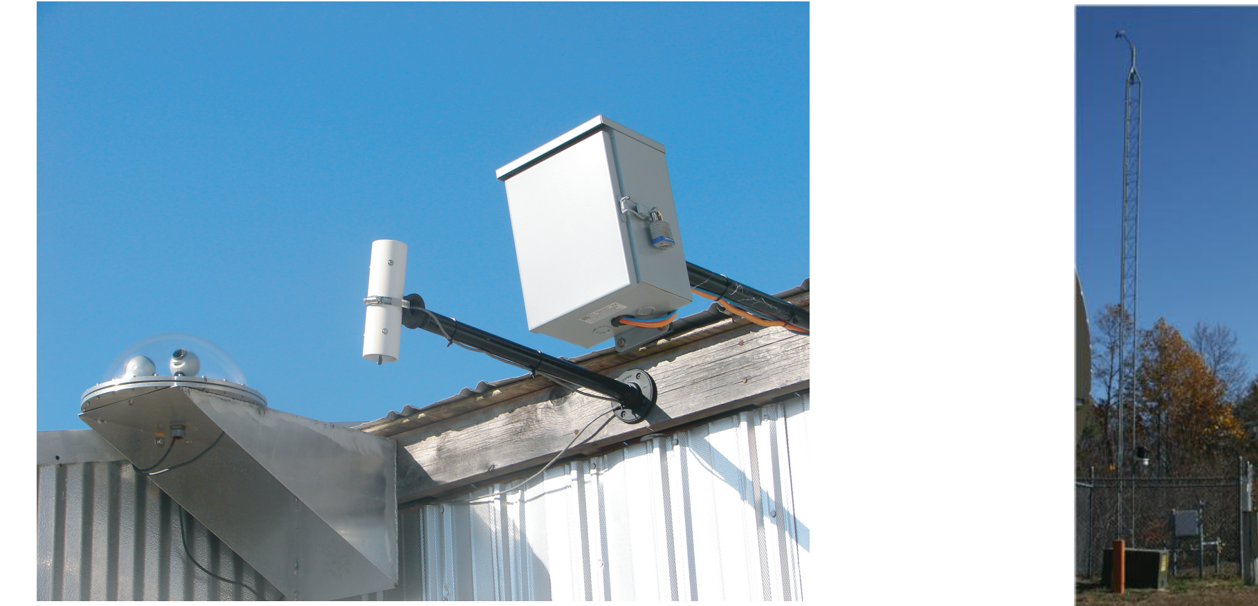
Figure 5: (Left to Right): SE and SW SkyCams, Cloud Sensor, and IR SkyCam. Right photo: Davis weather station and tower.
