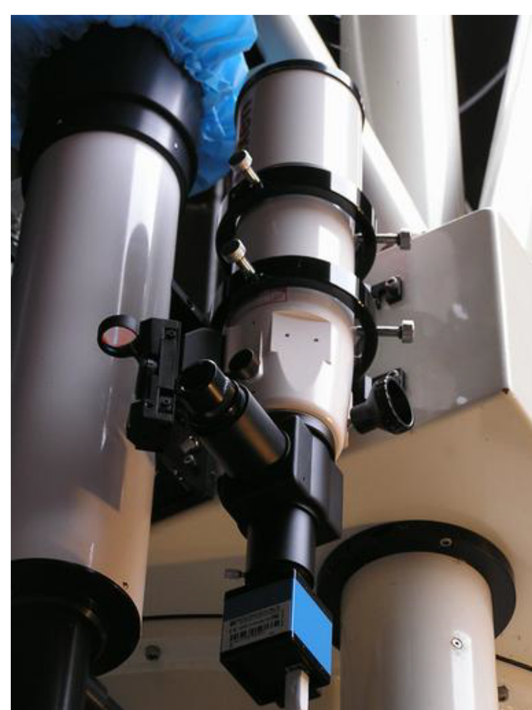
Figure 1: ImagingSource Finder Camera on Vixen Finder Scope
