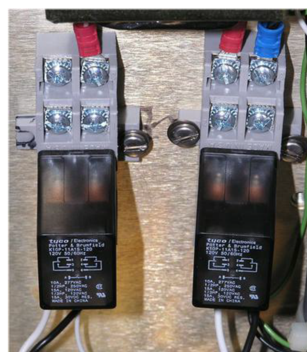
Figure 3: X10 Module-Controlled AC Relays
